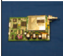
Trimble GPS Engine and Satellite Beacon Receiver for sub-metre accuracy Part # CTL-9201-0118
